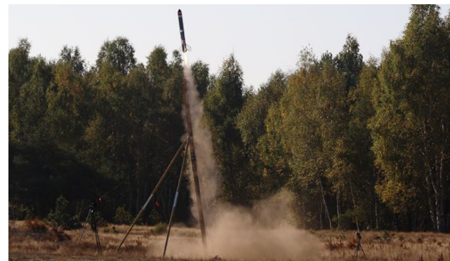
Figure: Mid-launch image of the Łukasiewicz - Institute of Aviation RDRE powered Rocket [1]
