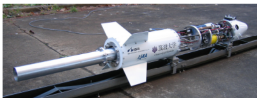
(a) PDE Powered Rocket from Kasahara [18]
