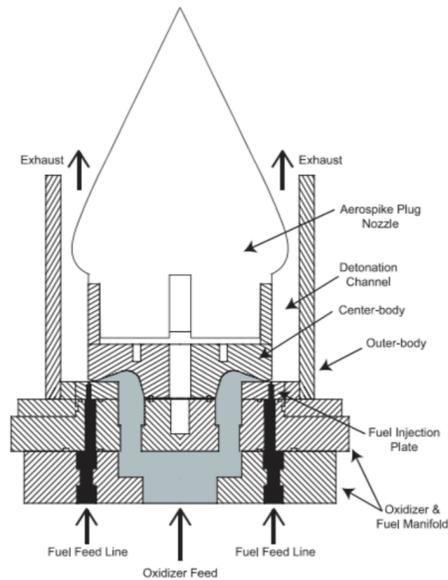
*Figure 6: Cross section of a typical RDE [16]*
