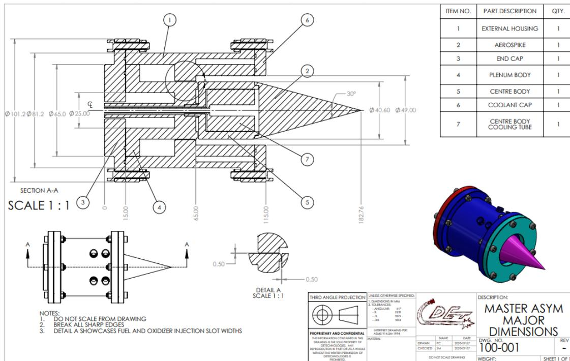
Figure 7: High-level assembly drawing depicting the major components and dimensions of the initial RDE geometry.
