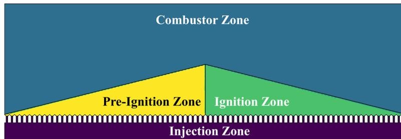
**Figure 9:** 2-D RDE Simulation Zone Identification [37].
